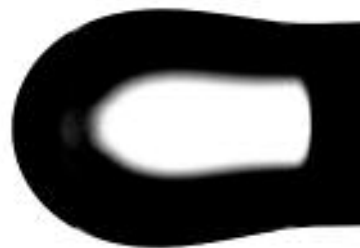
Fig. 2: Pendant drop of a hotmelt at 120^\circ\text{C}
